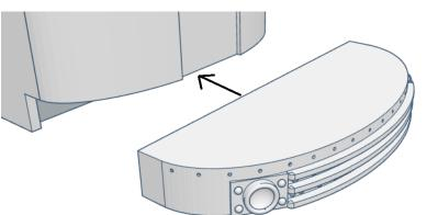
Adding the Scribed Siding: To complete the main assembly, obtain one sheet of 6" x 12" Evergreen Styrene O Scale Passenger Car Siding (item no 3047, 2–1/4 spacing, 030" thick). Cut pieces to fit each side panel, from the end of the side door top to just before the curve on the ends as shown by the lines below. These pieces should fit flush with the bottom of the side, and butt up against the side door and the letterboard. These can be laminated to the body using the adhesive of your choice.
