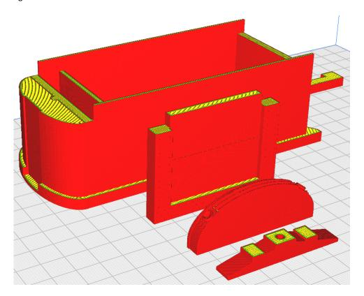
**Assembly:** Start the assembly by placing the two side halves on top of the floor plate. Orient the two side pieces so the letter-boards are at the top and interlock as shown in the picture below to leave the proper space for the side door panel. They should fit flush with the bottom of the floor.
