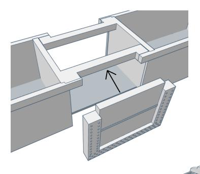
The bolsters can be glued to the underside of the frame where the two flat places are. Holes can be drilled and tapped for screws to hold the trucks in place.
