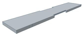
The roof is 324mm and may tax some smaller FDM printers. You can slice it in half for printing and then glue the two halves back together. Print the roof flat on the build plate.
