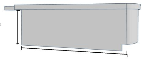
Cut four pieces to fit the end curved section. These pieces should sit flush on top of the anti-climber and butt up to the letterboard at the top, leaving the door opening clear. I recommend warming the plastic (hot water or heat gun) and wrapping it around a 1-2" diameter pole/bottle and letting it cool in that position. That will make it easier to conform to the curve. If you are modeling the version without the end door, just cut one piece long enough to wrap around the whole end.
