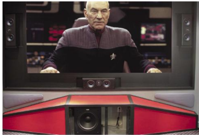
SOUND TREK ARRAY Three Polk CSi speakers flank the home-built screen, while a powered Velodyne CHT-12 subwoofer fires from the stage below.
