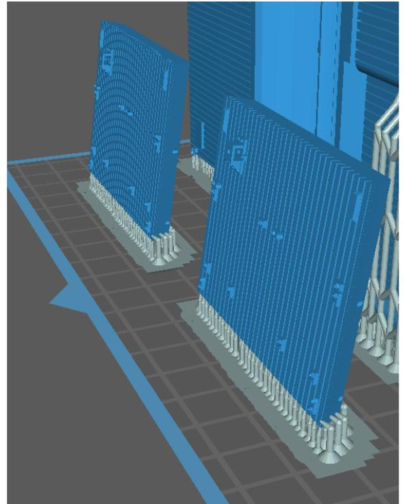
Use a lot of supports around the perimeter of the two body pieces to ensure they come out as flat as possible to aid in connecting the two halves together. Additional material was provided so they can be sanded flat without losing any of the model. See the next page for more details.
