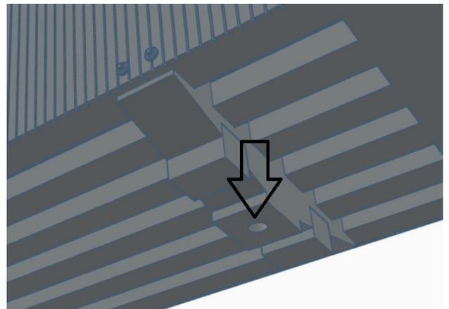
A model of a K Type brake cylinder is provided to detail the underbody. It is mounted in the center of the underframe between the two middle beams. See photo on next page.
