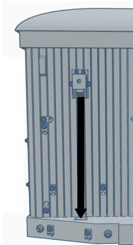
The brake wheel is installed in the hole on the mount. They may need to be drilled out to make a good fit.
