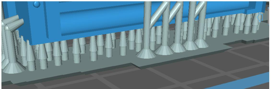
The brake wheels are best printed face down as shown here.
