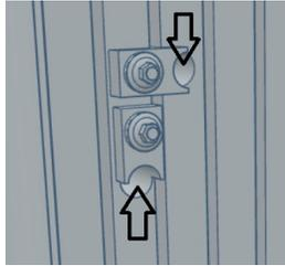
The holes may have to be drilled out in case they were filled with resin during the printing process. They should accept a .020 sized brass rod which is bent into a 'U' shape as shown here.
