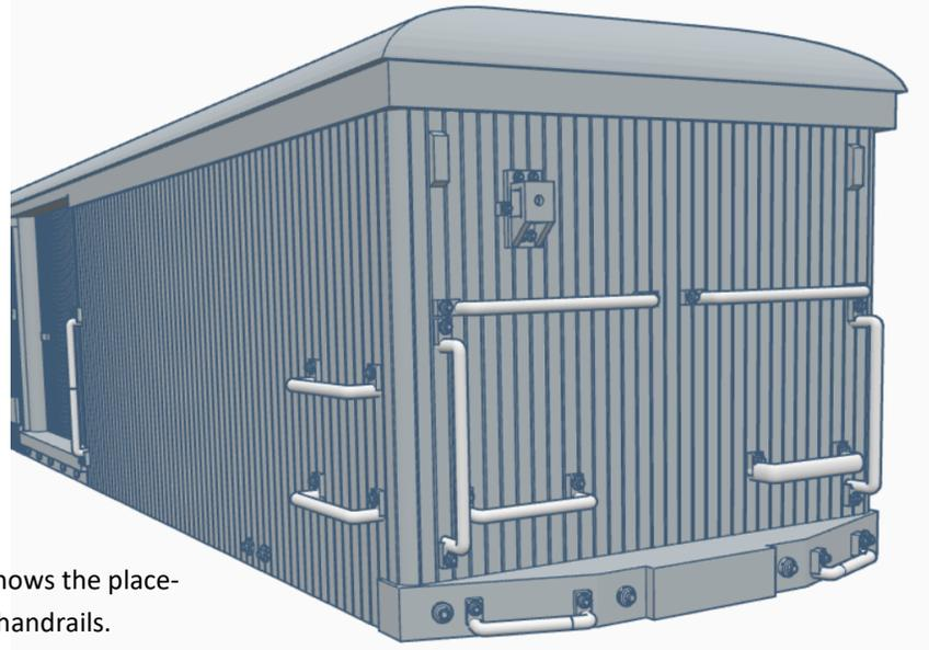
This photo shows the placement of the handrails.
