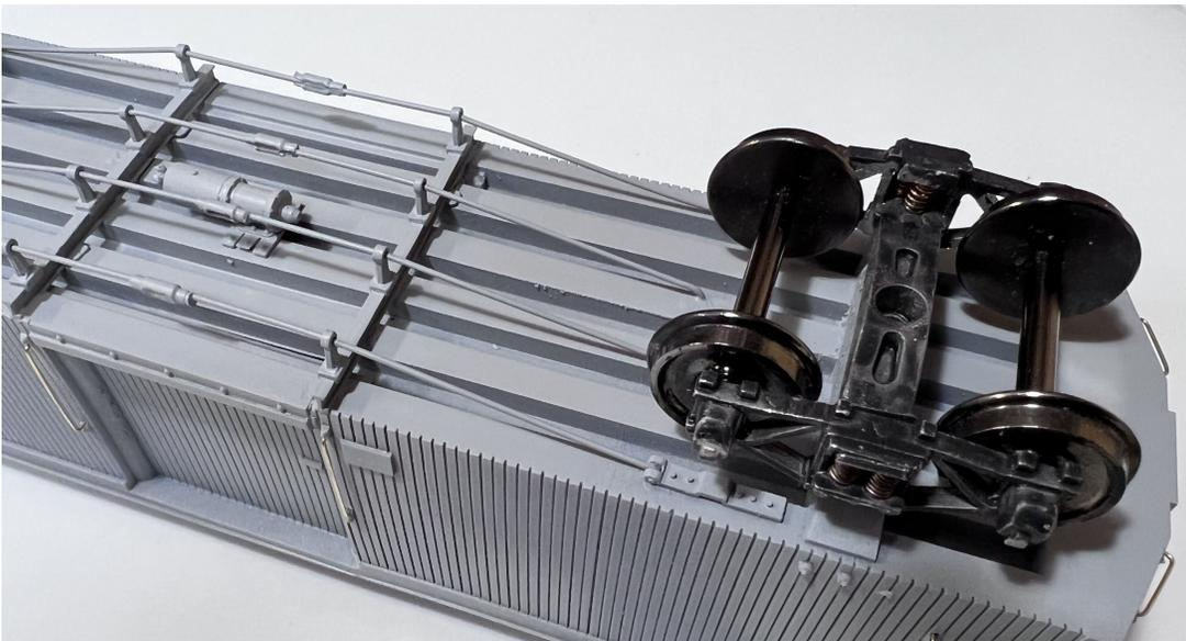
**Finishing:** As with any model there is an unlimited number of options for finishing. I recommend a fine surface primer (e.g. Tamiya Fine Surface Primer) be used to avoid masking the details. Refer to prototype photos for the details, color and decal placement.
