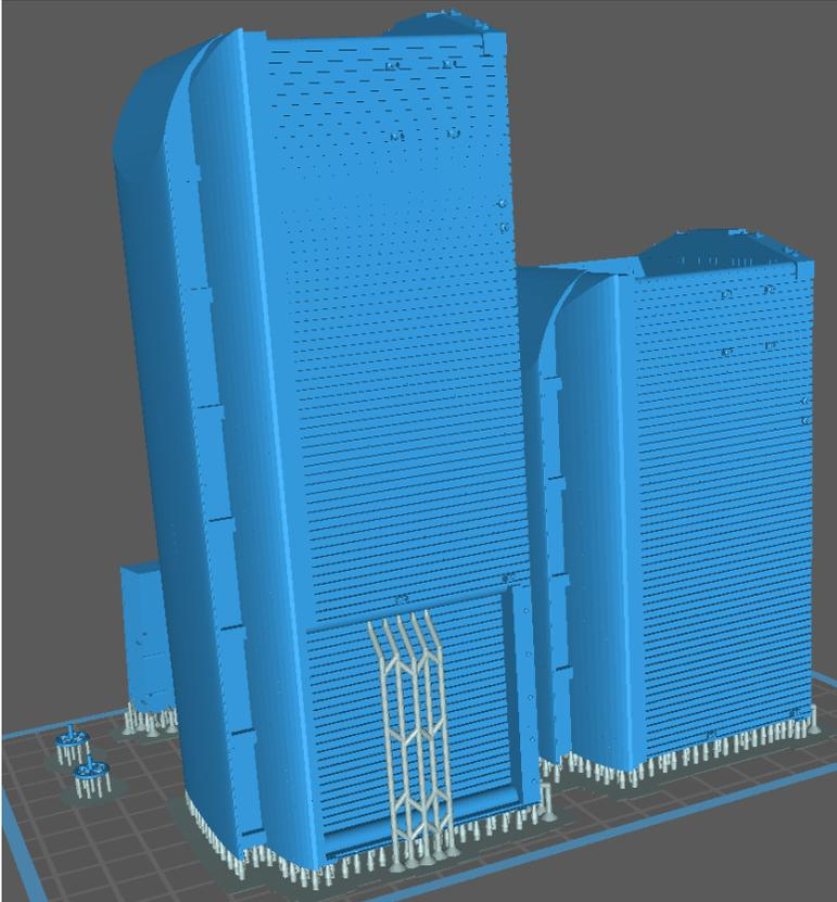
The two end pieces can be printed angled back slightly to minimize supports needed.
