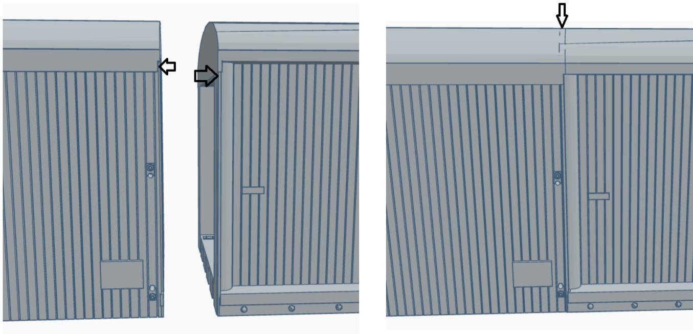
The end pieces are designed to be slightly larger so they can be sanded for a seamless fit. Make sure the mount for the brake wheel is at the top and is over the open slot on the bumper for the brake chain to hang through as shown by the arrow. Only one end has the brake wheel mount and opening in the bumper.
